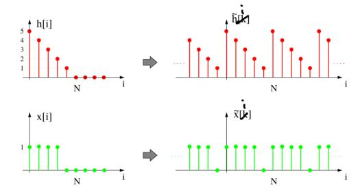
Multiplication in the time-domain leads to circular convolution in the frequency domain:
