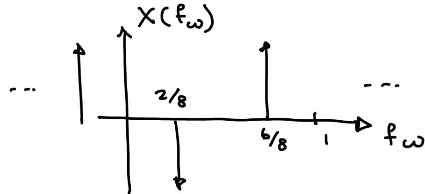
$$f_{\omega_0} = \frac{2}{8} = \frac{1}{4} \text{ [cycles/sample]}$$
