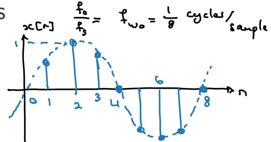
$$\frac{f_0}{f_s} = f_{\omega_0} = \frac{1}{8} \text{ cycles/sample}$$
